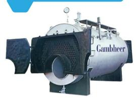
This package boiler comes in dry back, Semi-wet back & fully wet-back options. Package boiler work on solid fuel like coal, briquettes or wood. The furnace of the boiler is completely submerged in water. The three pass package boiler It is a conventional 3 pass smoke-tube design.
